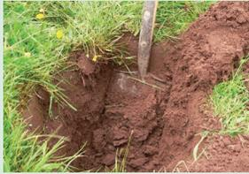
A well-structured and free-draining soil has abundant air spaces enabling water to percolate through soil. Surface-water runoff is unlikely on these soils.
